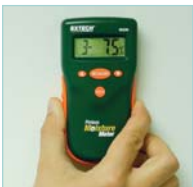
Measure moisture of wall material with non-invasive Pinless technology
