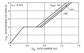
Figure 7. Gate Charge Characteristics.
