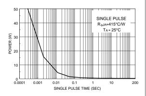
Figure 10. Single Pulse Maximum Power Dissipation.
