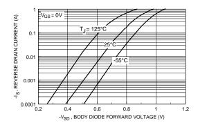
Figure 6. Body Diode Forward Voltage
