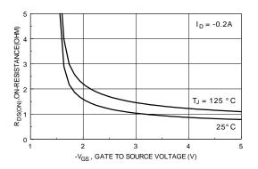
Figure 4. On-Resistance Variation with Gate-to-Source Voltage.
