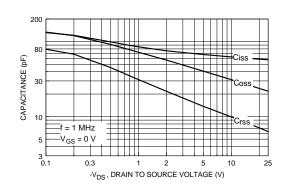
Figure 8. Capacitance Characteristics.
