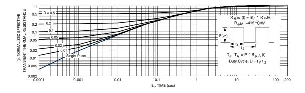
Figure 11. Transient Thermal Response Curve.
