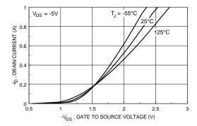
Figure 5. Transfer Characteristics.
