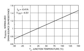
Figure 3. On-Resistance Variation with Temperature.
