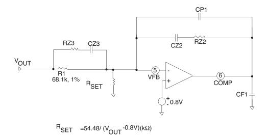
Type III Error Amplifier Compensation Circuit
