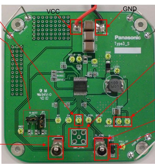
SMA\_SYNC (BNC terminal for external clock)
