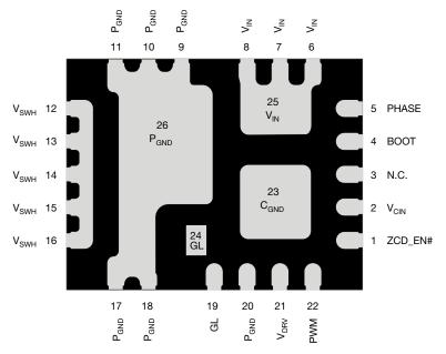
Fig. 2 - SiC534 Pin Configuration
