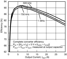
Fig. 8 - Efficiency vs. Output Current (V<sub>IN</sub> = 9 V)
