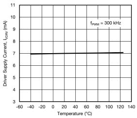
Fig. 16 - Driver Supply Current vs. Temperature
