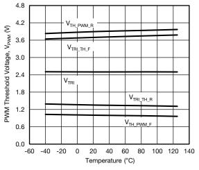
Fig. 14 - PWM Threshold vs. Temperature
