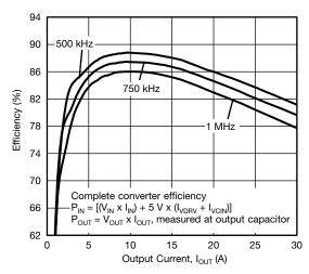
Fig. 11 - Efficiency vs. Output Current (V<sub>IN</sub> = 19 V)
