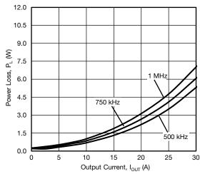
Fig. 10 - Power Loss vs. Output Current (V<sub>IN</sub> = 12.6 V)
