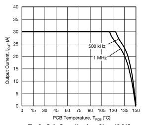
Fig. 9 - Safe Operating Area (V<sub>IN</sub> = 12.6 V)
