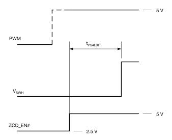
Fig. 5 - ZCD\_EN# - PS4 Exit Timing
