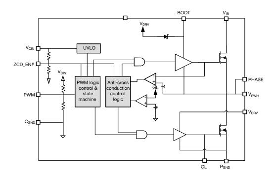
Fig. 3 - SiC534 Functional Block Diagram
