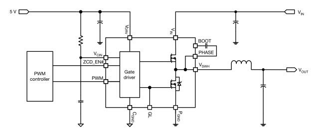
Fig. 1 - SiC534 Typical Application Diagram
