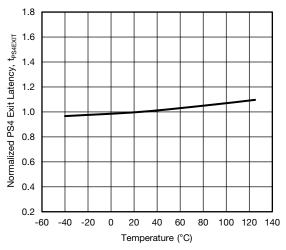
Fig. 15 - PS4 Exit Latency vs. Temperature
