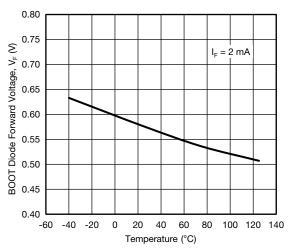
Fig. 13 - BOOT Diode Forward Voltage vs. Temperature
