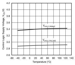
Fig. 12 - UVLO Threshold vs. Temperature
