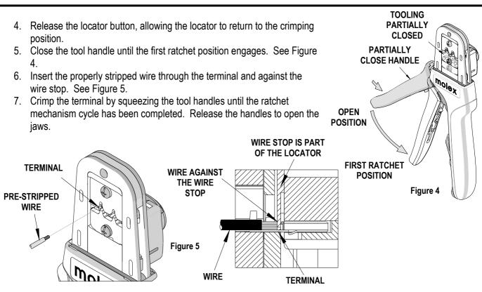
Note: The tamper proof ratchet action will not release the tool until it has been fully closed.
