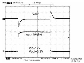
Figure 4. Load Step Response: 0->3A
