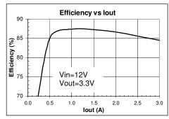
Figure 1. Efficiency Vs Load
