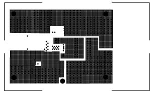
Figure 11. PCB Layout 3rd Layer Side
