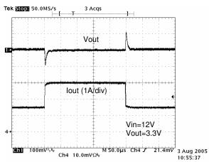
Figure 3. Load Step Response: 1.5->3A
