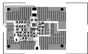
Figure 12. Bottom Side & Component Placement
