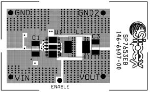
Figure 9. Top Side & Component Placement
