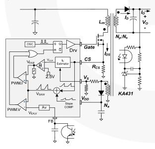
Figure 24. Internal PWM Control Circuit
