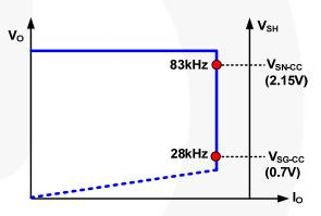
Figure 29. Frequency Reduction with V<sub>SH</sub>
