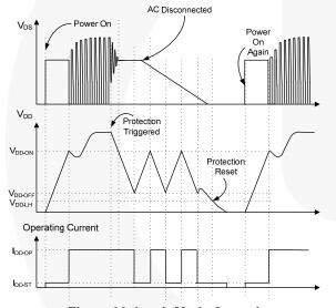
Figure 38. Latch-Mode Operation
