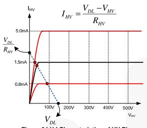
Figure 34.V-I Characteristics of HV Pin
