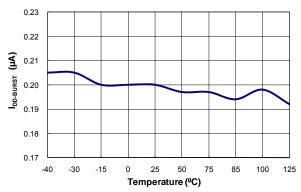
Figure 8. Operating Current (I<sub>DD-OP</sub>) vs. Temperature
