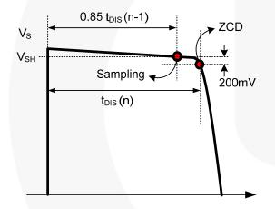
Figure 27. Detailed Waveform for ZCD
