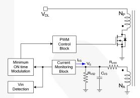
Figure 39. Vs Pin Current Sensing
