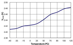
Figure 14. Reference Voltage of CS (V<sub>VR</sub>) vs. Temperature
