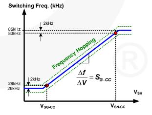
Figure 30. Frequency Reduction Curve in CC Regulation
