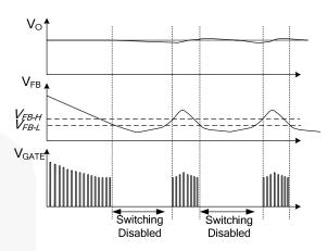
Figure 36. Burst-Mode Operation
