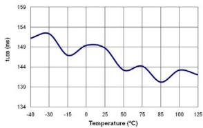
Figure 20. Minimum On Time (t<sub>MIN</sub>) vs. Temperature
