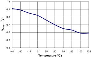
Figure 16. Starting Voltage of Frequency Decreasing Figure 17. Ending Voltage of Frequency Decreasing of of CC Regulation (V<sub>SN-CC</sub>) vs. Temperature CC Regulation (V<sub>SG-CC</sub>) vs. Temperature
