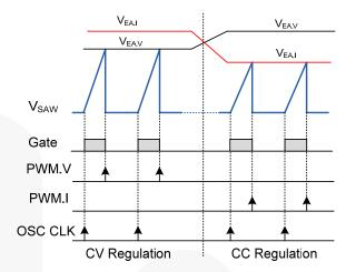
Figure 25. PWM Operation for CC and CV
