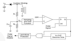
Figure 41. V<sub>S</sub> OVP Protection
