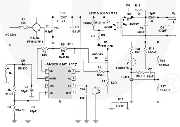
Figure 43. Schematic of Typical Application Circuit
