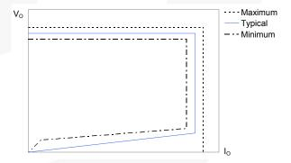
Figure 1. Typical Output V-I Characteristic
