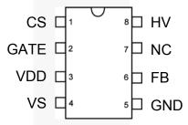
Figure 5. Pin Assignments
