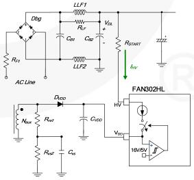
Figure 33. HV Startup Circuit
