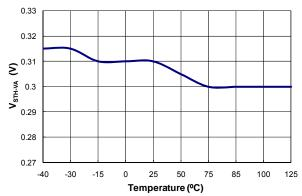
Figure 18. Threshold Voltage for Current Limit (V<sub>STH</sub>) vs. Temperature
