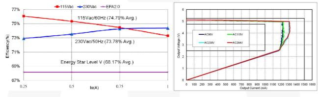
Figure 42. Measured Efficiency and Output Regulation
