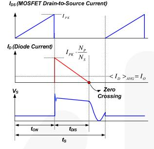
Figure 26. Key Waveforms of DCM Flyback Converter
