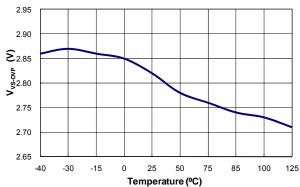
Figure 12. Leave Zero Duty Cycle of FB Voltage (V<sub>FB-H</sub>) vs. Temperature
