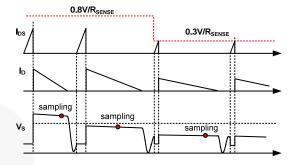
Figure 32. Power Limit Mode Operation
