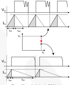
Figure 28. t<sub>DIS</sub> Variation in CC Mode
