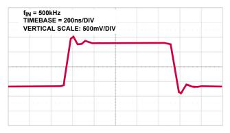
FIGURE 11. LARGE SIGNAL STEP RESPONSE
