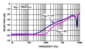
FIGURE 6. PSRR vs FREQUENCY
