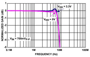
FIGURE 2. LARGE SIGNAL GAIN vs FREQUENCY -0.1dB
