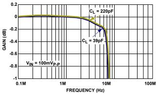
FIGURE 4. GAIN vs FREQUENCY FOR VARIOUS CLOAD
