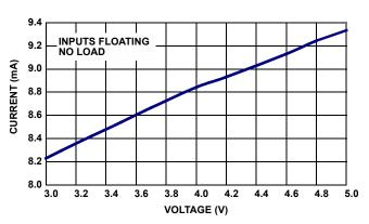
FIGURE 10. SUPPLY CURRENT vs SUPPLY VOLTAGE
