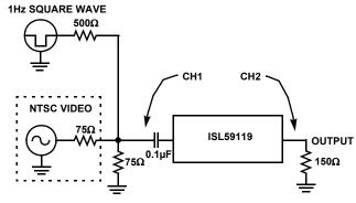
FIGURE 27. DC STEP RESPONSE CIRCUIT
