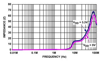
FIGURE 7. OUTPUT IMPEDANCE vs FREQUENCY
