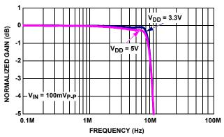
FIGURE 1. SMALL SIGNAL GAIN vs FREQUENCY -0.1dB
