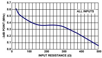
FIGURE 22. -3dB BANDWIDTH vs INPUT RESISTANCE
