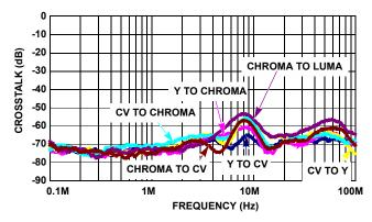
FIGURE 8. CROSSTALK vs FREQUENCY
