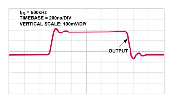
FIGURE 12. SMALL SIGNAL PULSE RESPONSE
