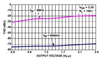
FIGURE 20. TOTAL HARMONIC DISTORTION vs OUTPUT VOLTAGE
