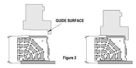
Using the application tool and an appropriate press, seat the Daughtercard module until there is less than 0.10mm (.004 in) clearance between the bottom of the plastic housing and the surface of the PCB. See Figure 3.
