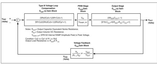
SP7655 Voltage Mode Control Loop with Loop Dynamic
