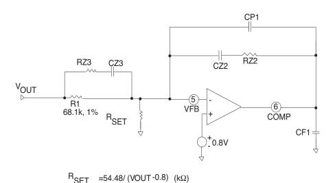
Type III Error Amplifier Compensation Circuit
