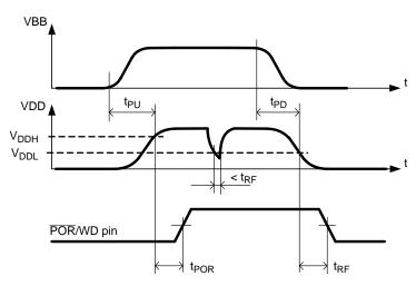
Figure 14. Power-on-Reset Timing Diagram
