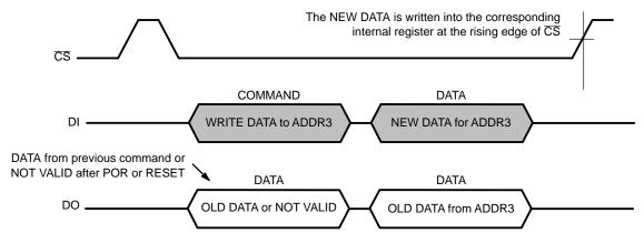
Figure 19. Single WRITE Operation where DATA from the Master is Written in SPI Register with Address 3
