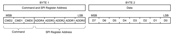
Figure 17. SPI Transfer Packet
