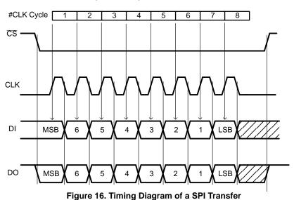
NOTE: At the falling edge of the eighth clock pulse the data–out shift register is updated with the content of the addressed internal SPI register. The internal SPI registers are updated at the first rising edge of the NCV70522DQ system clock when  $\overline{CS}$  = High.
