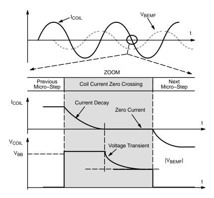
Figure 12. Principle of Bemf Measurement
