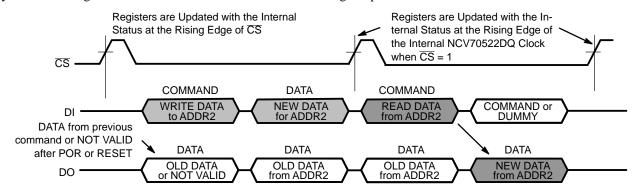
Figure 21. A WRITE Operation where DATA from the Master is Written in SPI Register with Address 2 Followed by a READ Back Operation to Verify a Correct WRITE Operation
