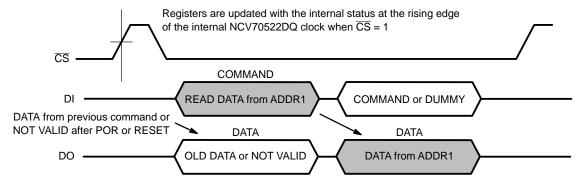
Figure 18. Single READ Operation where DATA from SPI Register with Address 1 is Read by the Master
