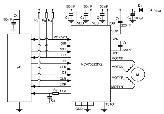
Figure 5. Typical Application Schematic NCV70522DQ
