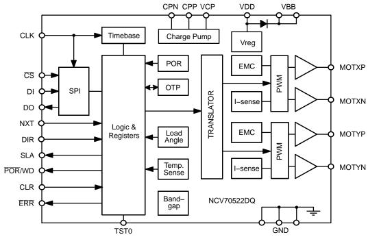
Figure 1. Block Diagram NCV70522DQ
