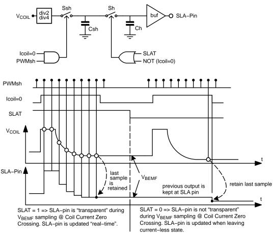
Figure 13. Timing Diagram of SLA-Pin
