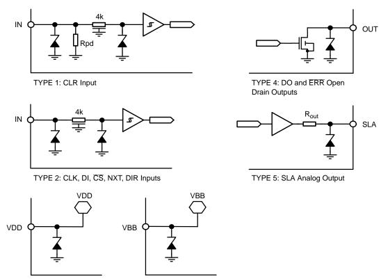
TYPE 3: V<sub>DD</sub> and V<sub>BB</sub> Power Supply
