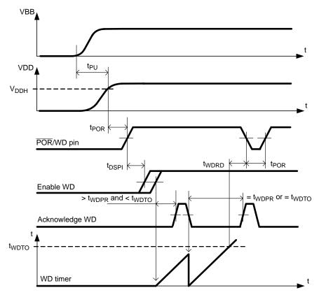
Figure 15. Watchdog Timing Diagram
