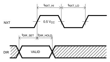
Figure 3. NXT-Input Timing Diagram
