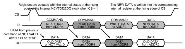
Figure 20. Two Successive READ Commands Followed by a WRITE Command
