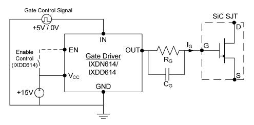
Figure 14: Recommended Gate Diver Configuration (Option #2)
