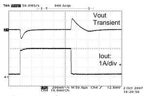
Figure 4. Load Step Response: 0.3A->3A
