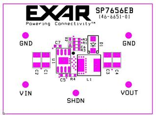
Figure 10. SP7656EB Top Side Component Placement
