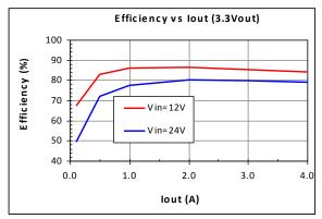
Figure 1. Efficiency vs. Load
