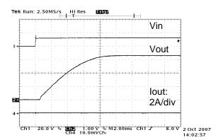
Figure 7. Startup No Load
