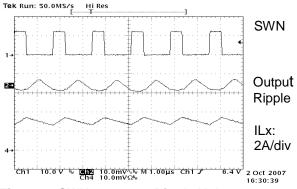
Figure 3. SWN & Output Ripple Voltage
