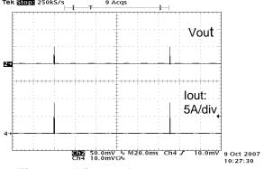
Figure 6. Hiccup due to overcurrent
