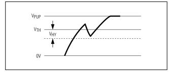
Figure 12. Hysteresis at the Low-to-High Switching Threshold
