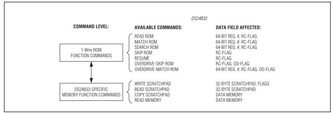
Figure 2. Hierarchical Structure for 1-Wire Protocol
