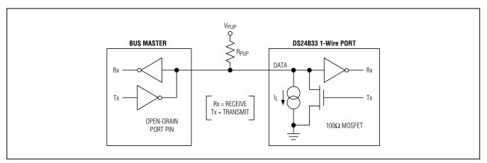
Figure 8. Hardware Configuration
