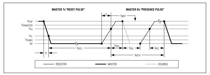
Figure 10. Initialization Procedure: Reset and Presence Pulse
