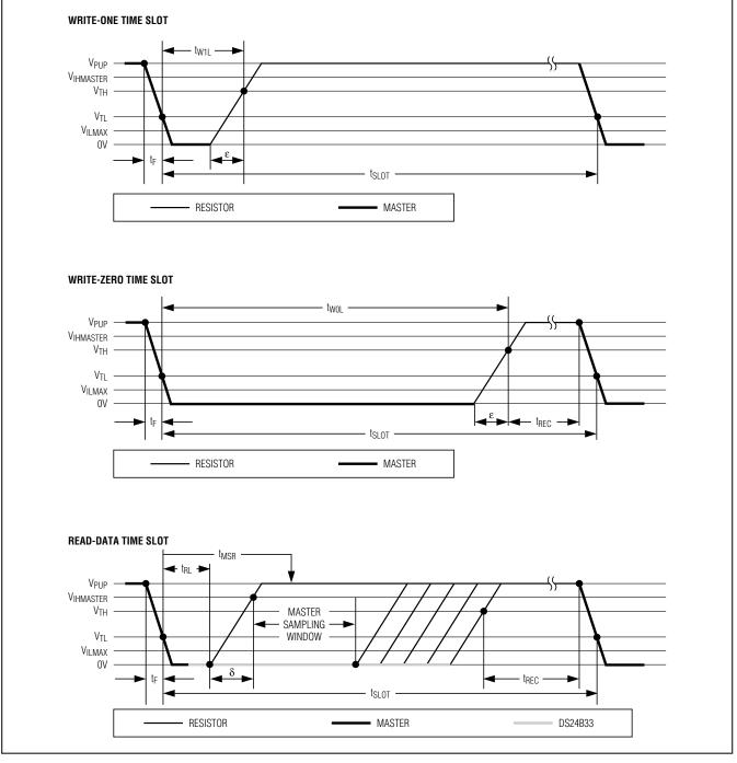
Figure 11. Read/Write Timing Diagrams
