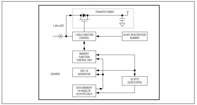
Figure 1. Block Diagram
