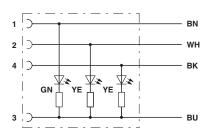
Contact assignment of M12 sockets with LED
