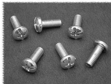
Part #: 1421D (package of 25) • 10-32 x 0.5" • Slotted & phillips combination pan head screws • Use where economy is important OR for close panel spacing. • Zinc plated
